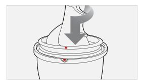
Note: The Ultrasqueezer needs to be locked in place in order to close the Hopper.
